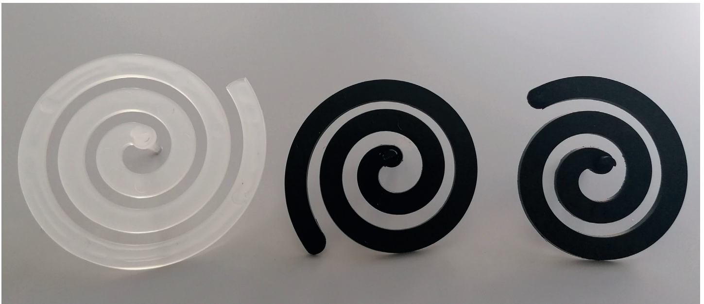
Fig. 3: Comparison of the achieved flow distance in the flow spiral tool with the same injection moulding conditions, starting on the left, of PP DuPure L50E, NEFA MB EL 23381S and NEFA MB EL21845S
