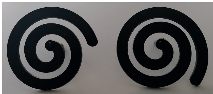
Fig. 6: Comparison of resultant flow distances in the same injection moulding conditions of NEFA MB EL 21845S. Left, standard, and right, with use of 2 % additive (NEFA MB A 19389)
